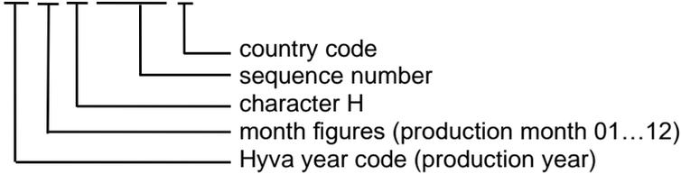
For Oil tanks; Guide arms; Hyfix; PTO's; casted and forged parts the convention is as follows:
